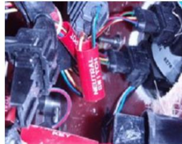
Neutral Switch (Helm Underside) view
